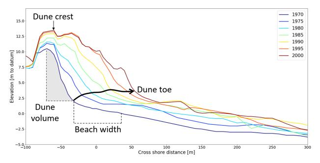
Example of characteristic parameters that can be extracted using the JAT.
